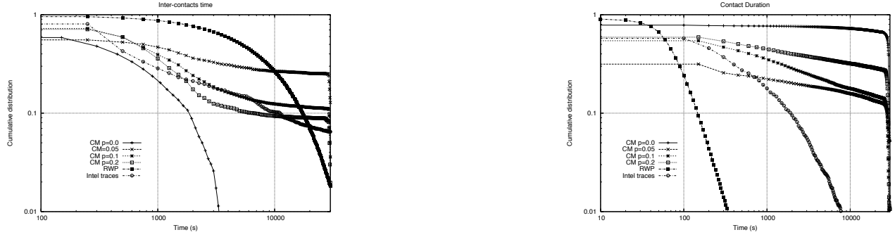
Figure 7: Comparison between synthetic and real traces (log-log coordinates) : (a) cumulative distribution of inter-contacts time in seconds; (b) cumulative distribution of contacts duration in seconds.
